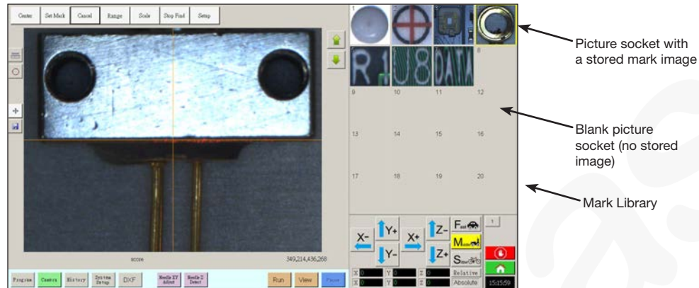
Camera screen shown in the Primary View screen and the Mark Library shown in the Secondary View screen
