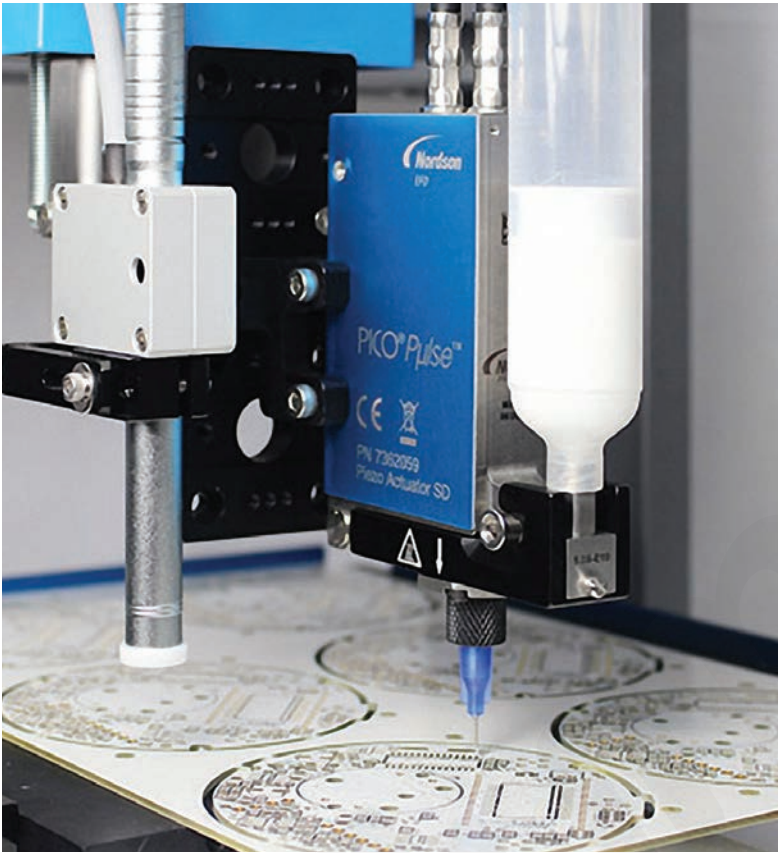
The PICO Pulse contact dispense valve provides precise, high-speed dispensing.
